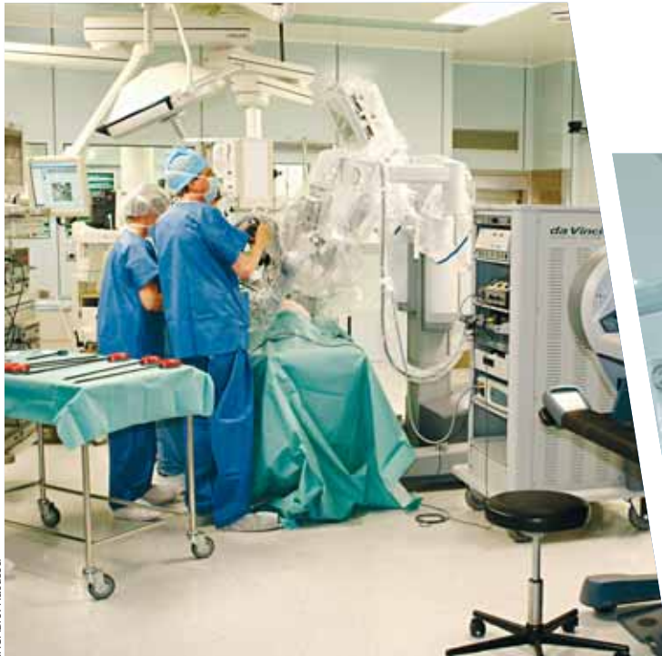
Intuitive Surgical's Da Vinci S robot features four jointed arms (one camera-based vision system, two operator arms, and one retractor arm). The camera, which can enlarge the images it captures up to 800%, allows surgeons to control the extremities of the robot's three-millimeter instruments, performing highly precise actions.
