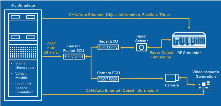
Figure 6: ADAS HIL Test Environment
