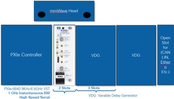
**Figure 7: 2-Target 1-Angle System Architecture**
