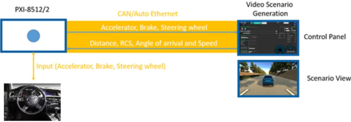
Figure 5: Vehicle communication Emulation
