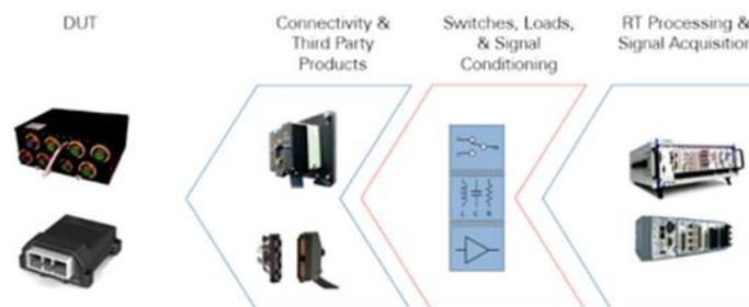
**Figure 9: How SLSC fits into an HIL system**
