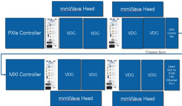
**Figure 8: 8-Target 4-Angle System Architecture**
