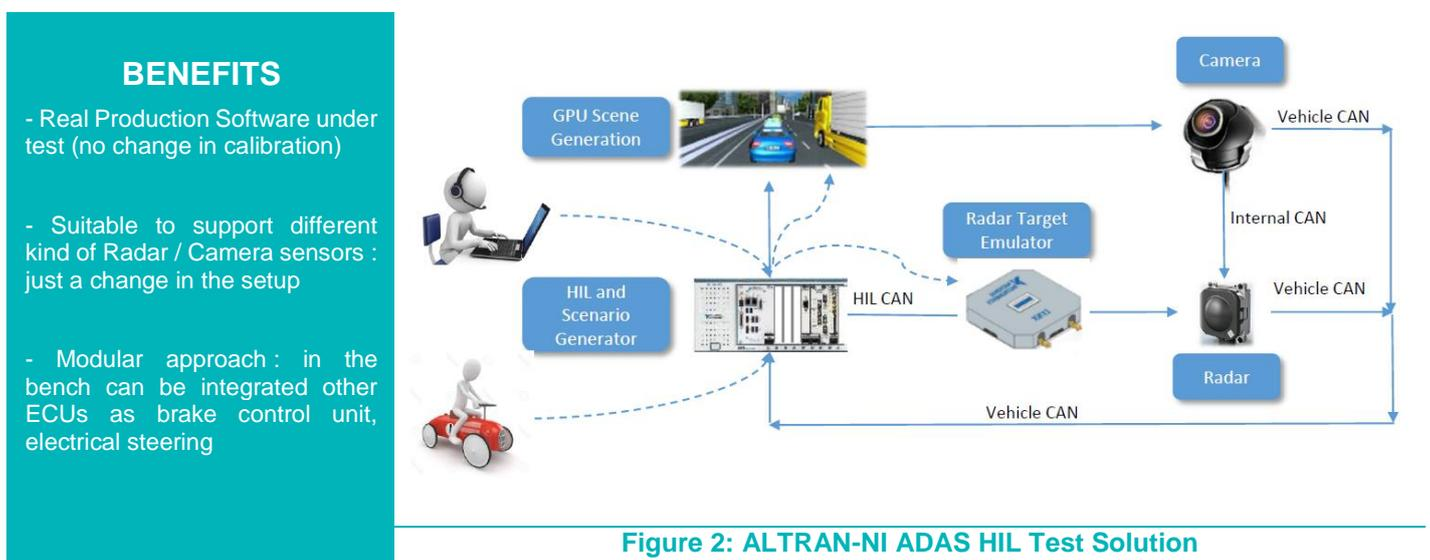
The 3D scenario is based on the Unity Graphic Engine and is fully configurable, including parameters like: number of lanes, lighting conditions, and track type are just a few of the things you can change.
